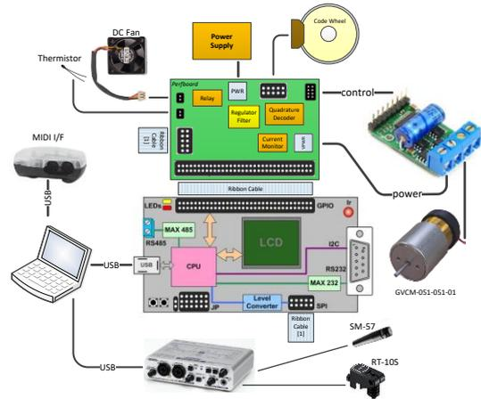
**Figure 9. Prototype Schematic.**
