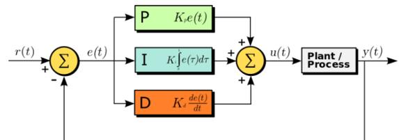
Figure 3. PID Controller.
