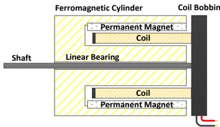
Figure 1. VCA Cutaway.
