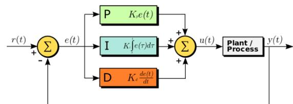
Figure 3. PID Controller.
