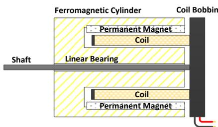
Figure 1. VCA Cutaway.
