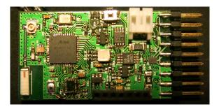
Figure 6: First prototype of the new wireless node.
