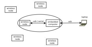
Figure 5: The setup for the new Sense/Stage system
