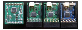
Figure 4: The different hardware revisions of the MiniBee; from left to right revision A, B, D and F.
