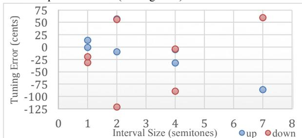
Figure 7. Accuracy of tuning mechanism performing different pitch intervals.
