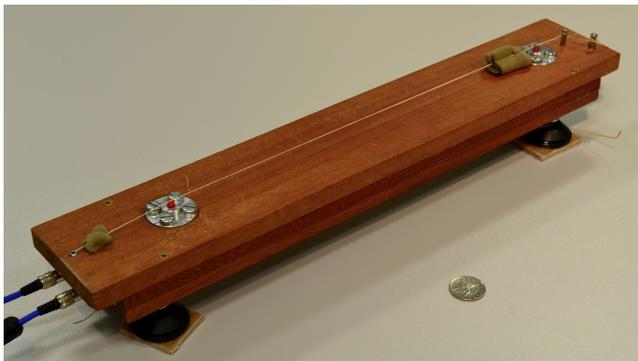
**Figure 3: The string-board controller.** The string is stretched over two bridge pistons, each of which rests on an internally mounted piezoelectric disk that sense the vibrations. Foam pieces are employed to suppress round-trip waves along the string.
