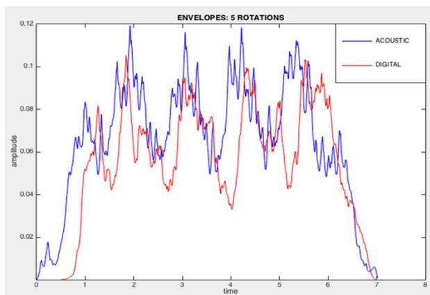
Figure 5: Envelopes for 5 Rotations of the Acoustic and Digital Wind Machines
