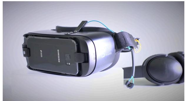
Figure 1. The VRHMD with an EEG attached and noise-canceling headphones
