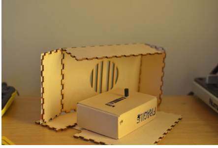
Figure 4: Nested boxes featuring a Laser-cut box “protecting” a cardboard box that encloses a metallic box carrying the fragile board.
