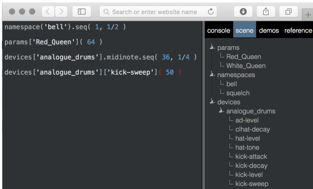
Figure 2: On the right, a treeview displaying the scene representing the patch shown in Figure 1 in the gibberwocky.max client. Users can drag and drop leafs from the tree into the code editor to insert paths for targeting specific devices / parameters, as seen at left.
