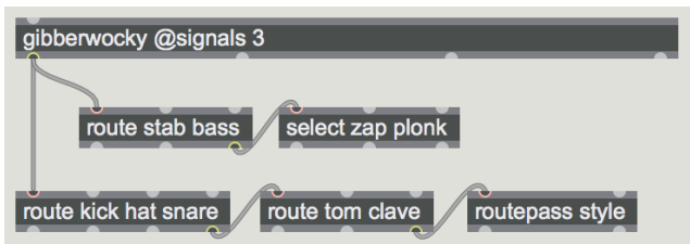
Figure 3: An example of routing messages (as opposed to signals) from the gibberwocky object for Max/MSP. When the patcher is saved, all of “stab”, “bass”, “zap”, “plonk”, “kick”, “hat”, “snare”, “tom”, “clave”, and “style” will be automatically included in the client’s derived namespace.
