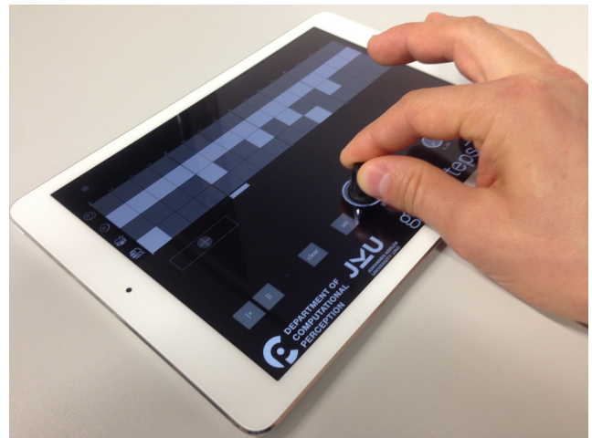
Figure 4: A physical knob used to control the variation dial on the touch surface. While the used knob is an improvised prototype, commercial products already exist for this purpose.
