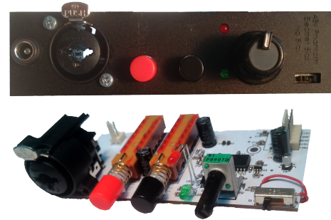
Figure 3: The custom preamp used to condition the audio signal. Top: Behind a panel, Bottom: Bare circuit board.
