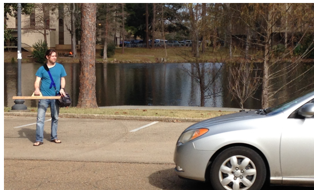
Figure 6: Portable eight-channel microphone array being used to record the sound wave field created by a car driving by.
