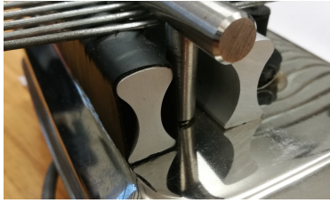
Figure 2. Insulated capacitive-sensing bridge (left).
