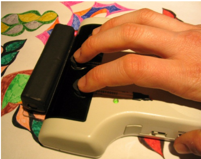
Figure 1. The Sonic Scanner is a new instrument for music performance that turns drawings, pictures, etc. into sound.
